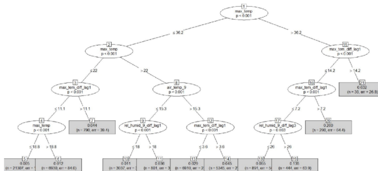
Figure 60 Partitioning of asset failure fires based on the contribution of different environmental factors
