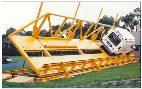
Figure 10 The tilt deck for testing articulated vehicles, installed at the ARRB site in 1984 (removed c2002). Source: ARRB 1993
