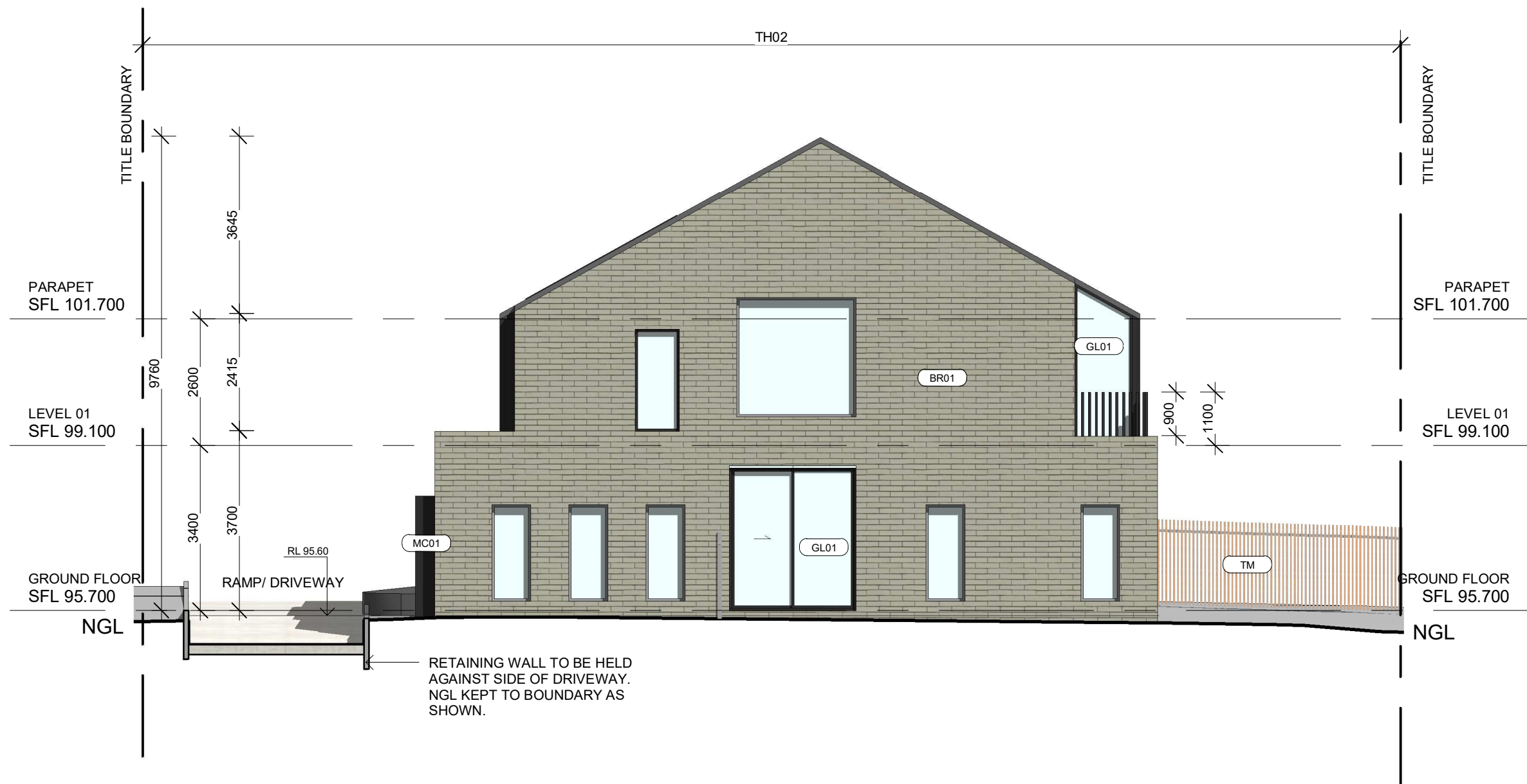
2 ELEVATION INTERNAL NORTH TP0.11 SCALE 1: 100
